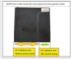
80FWNX Photo of rubberized handrail after rubbing with alcohol
